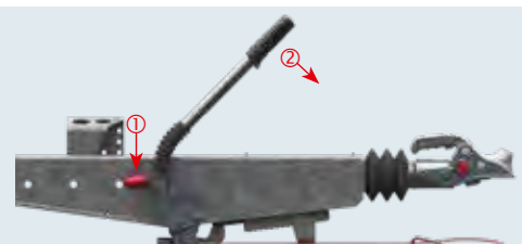
Handbrake lever applied = brake rod clamped
