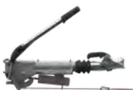
Handbrake lever closed (parking brake forwards)
