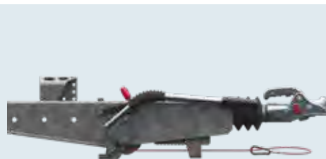
Handbrake lever opened = brake rod not clamped
