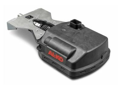
The caravan's driving response is continuously monitored by the ATC. Sensors detect dangerous lateral movements directly on the caravan axle, before any ESP system for trailers installed in the car is even able to sense the pendulum movement. The caravan will immediately — without any action on the part of the driver — brake gently and return to a stable driving condition.
